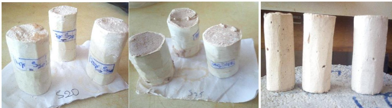
Figure 9: Curing test of the specimens at different percentage of lime and metakaolin
