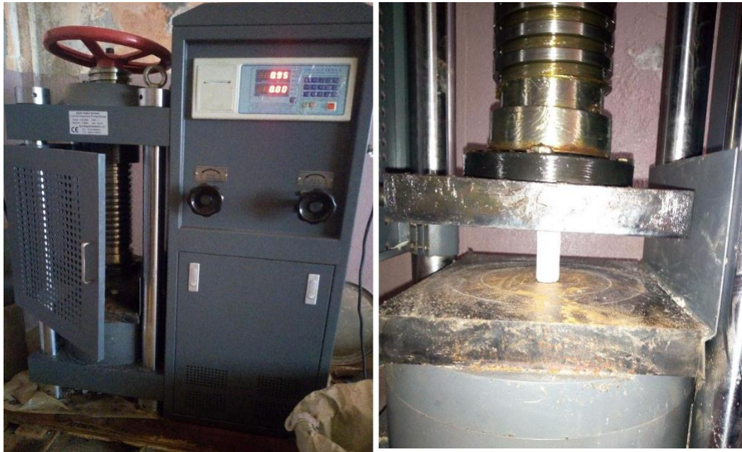
Figure 11: Compression of the specimens with the electric crusher
