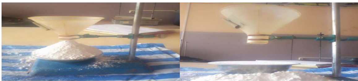
Figure 6: Apparent density Test process
