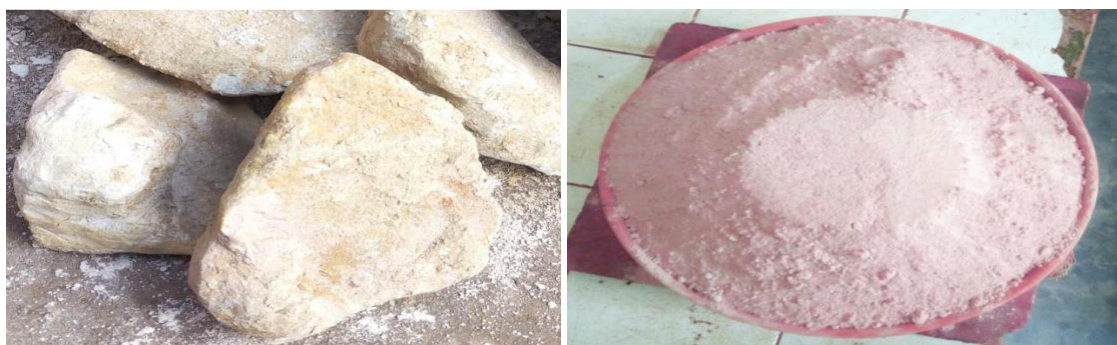
Figure 13: Hallosyte Balengou clay at it raw state and at 750°C after crushing.
